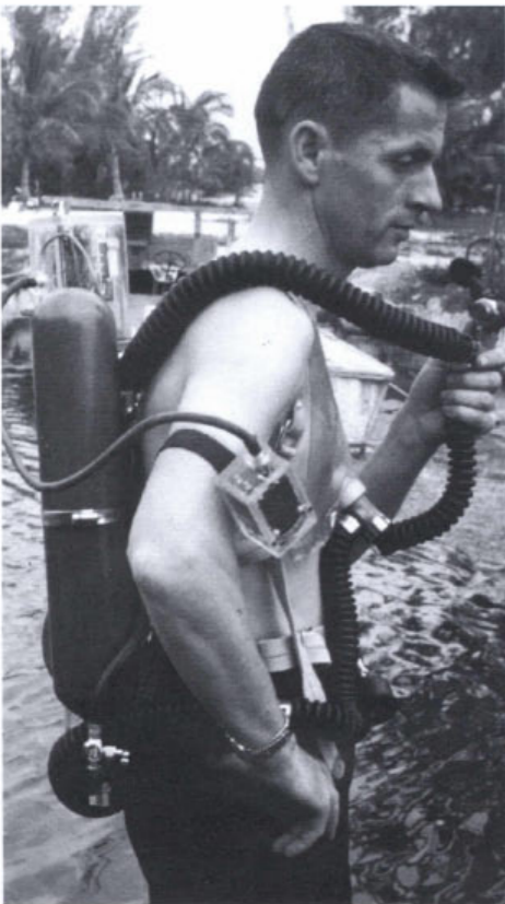
Developed in the late sixties, the Electrolung, an early predecessor to the Biomarine CCR 1000 was the first commercially available, electronically controlled, closed circuit mixed gas diving apparatus.
