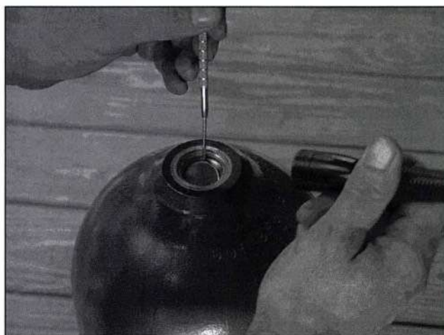
Inspecting for neck cracks using a penlight and magnifying mirror
