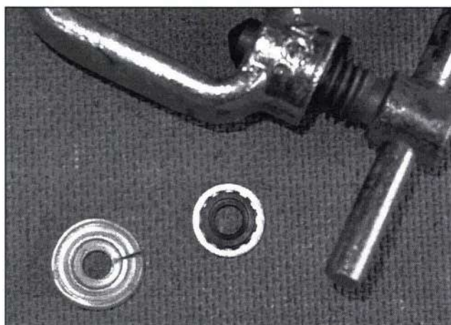
Hard plastic washer, somewhat the worse for wear, and a Bodok seal.
