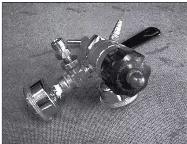
Medical regulator with a DISS port added to the LP port to take a demand mask
