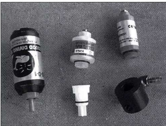
Sensors and related hardware. Pequot with built-in hose barb, Teledyne R17 MED with "flow diverter" and Maxtec CAG250 with "concentrator".
