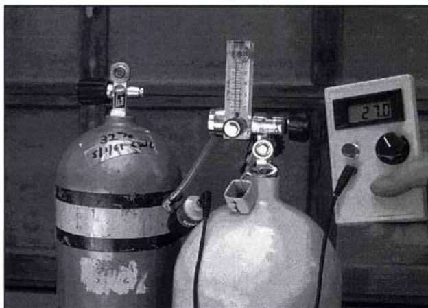
Analyzing a mix using a flowmeter and a Maxtec concentrator..
