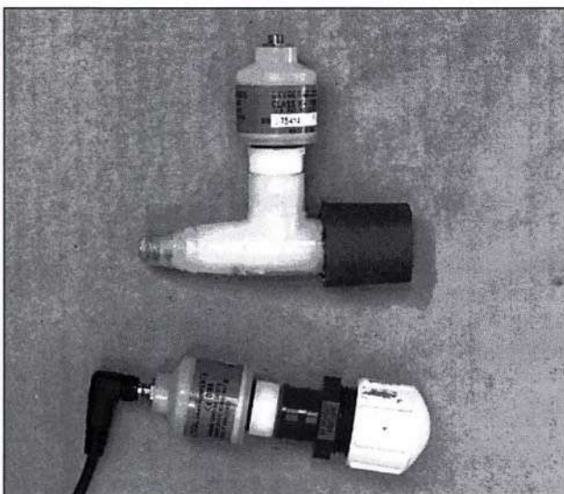
"Instant samplers" for direct-from-tank sampling. Hose tee at top, and Analox-style dome at bottom.
