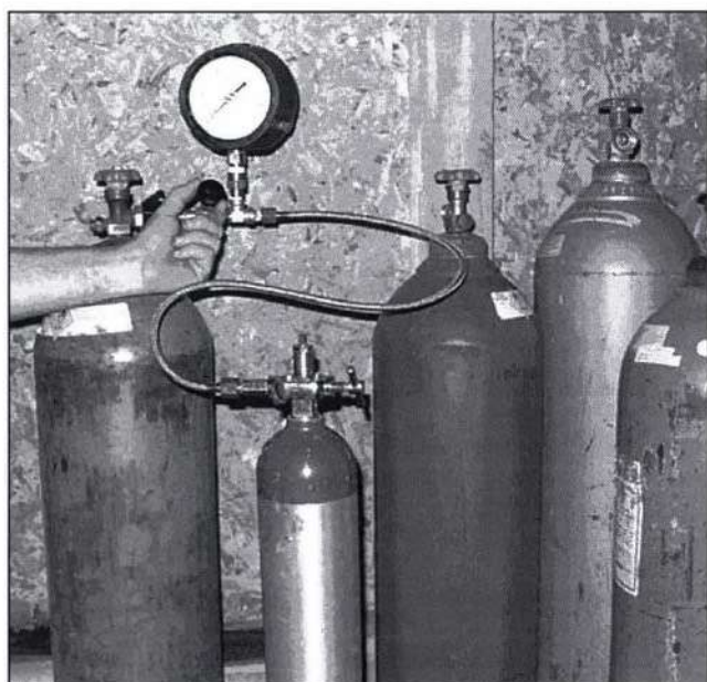
Good technique (and a reliable needle valve) are essential when filling small tanks
