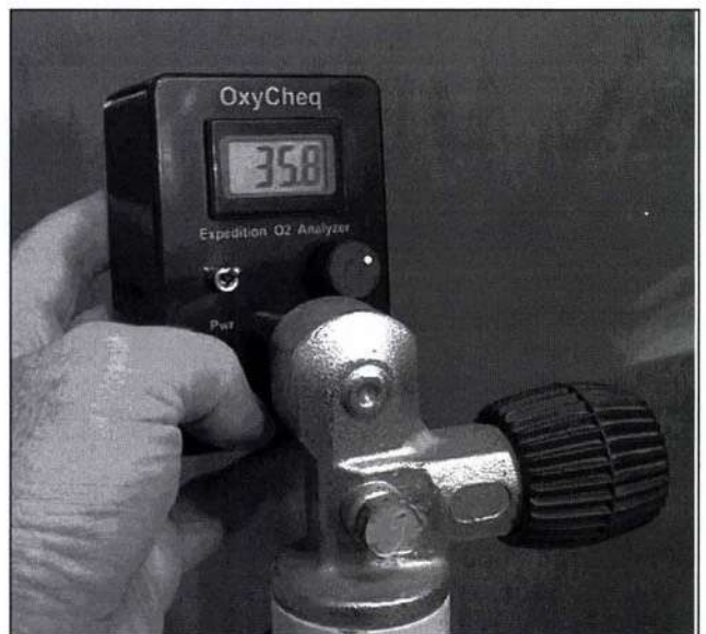
Oxycheq's Expedition analyzer reading directly from tank. Note the compact size.
