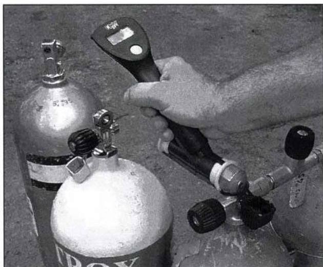
The OxySpy analyzer reads directly from the tank so no sampler is necessary.
