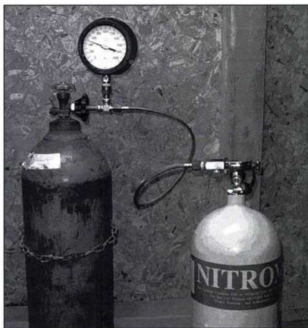
Partial pressure blending using a whip
