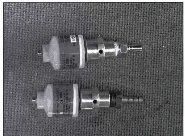
Two versions of the simple brass 3/6-1/4 adaptor concentrator, one with a hose barb and the other with a BC QR and flow restrictor
