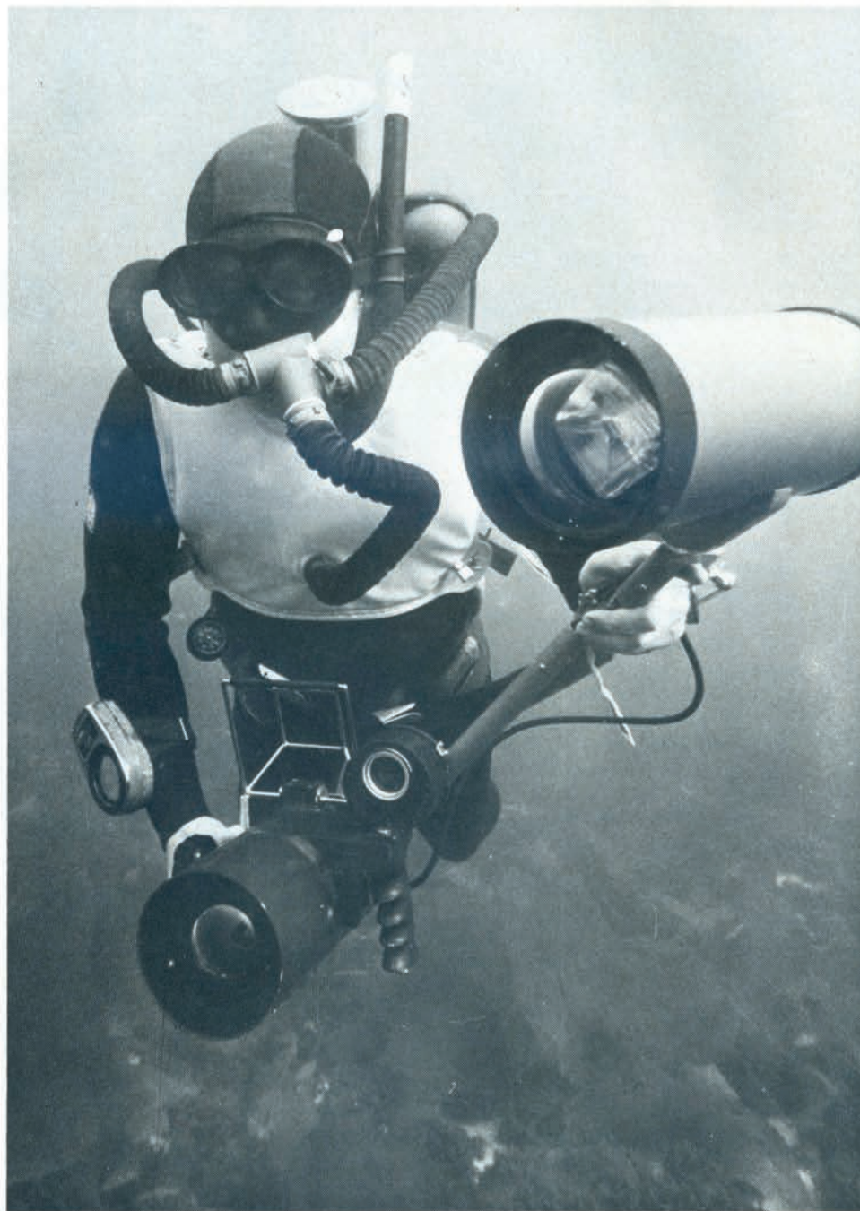
U/W photographer Bob Hollis checks out the Electrolung for cold water diving. At lower temperatures, the effective absorption time for baralyme is reduced.
