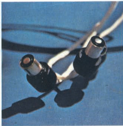
Thimble-sized electro-chemical sensors monitor the partial pressure of oxygen.
