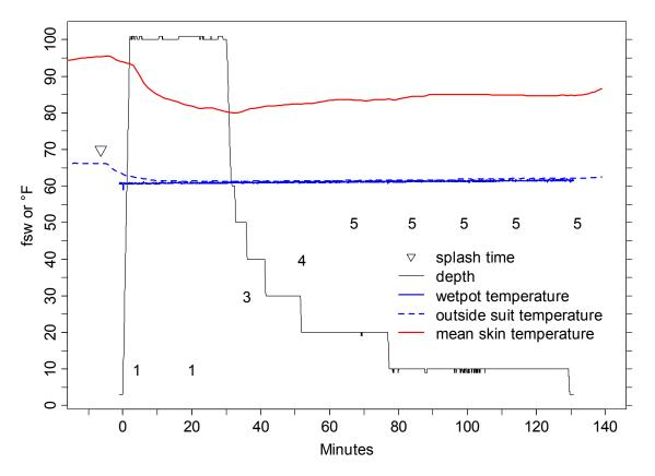
Figure F1. Typical depth-temperature-time record for wet-suited diver (Blue Diver, Team 2). Plotted numerals are the thermal status scores.
